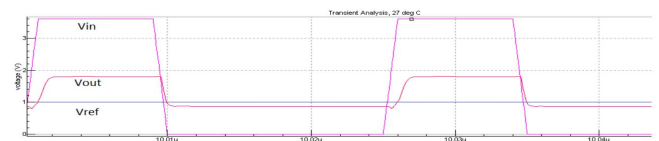
Fig. 6. Comparator waveform in v_{in}, v_{out} and v_{ref} .
