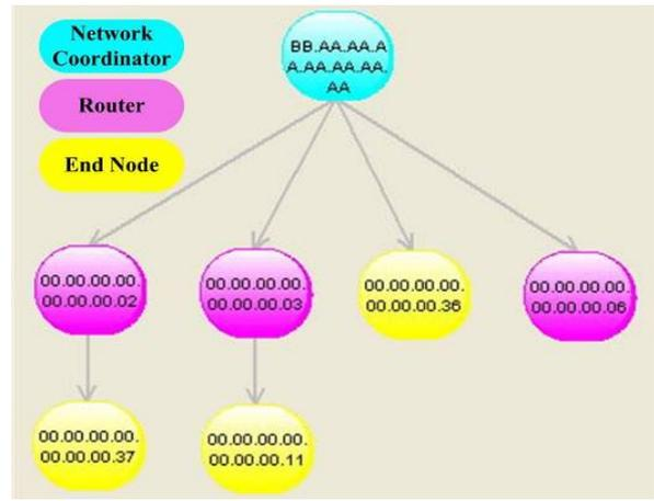
Fig. 7. ZigBee Network Topology of the Proposed System
