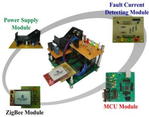
Fig. 6. Hardware Prototype of the Proposed Novel Fault Indicator
