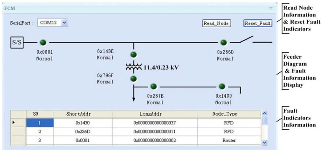
Fig. 5. HMI for the Fault Detection and Identification System
