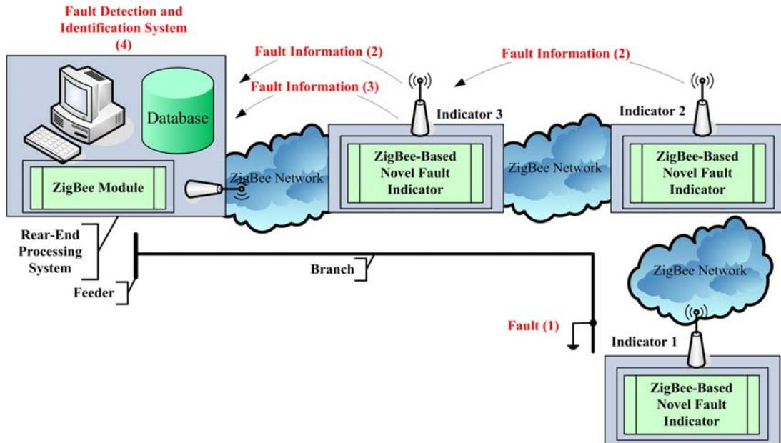
Fig. 4. Concept of the Fault Detection and Identification System
