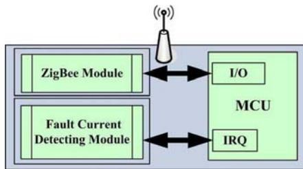
Fig. 1. Hardware Architecture of the Proposed Novel Fault Indicator
