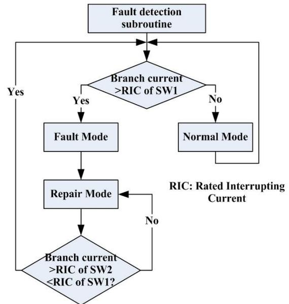
Fig. 3. Flowchart of Different Mode Exchange
