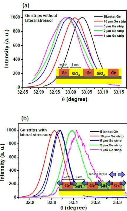
Fig. 7. High resolution XRD spectra for ge array (a) without and (b) with SiN lateral stressors. Insets show the cross-section schematics of the ge array strips.
