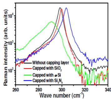
Fig. 4. High resolution Raman spectra of *n*-doped ge epi film with various capping layers.
