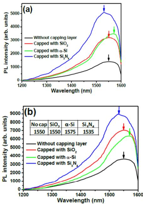
Fig. 3. (a) Directly measured PL spectra and (b) PL spectra after correction to the reflectance of pumping laser and light-out extraction efficiency of the P<sup>+</sup>-implanted ge samples annealed with various capping layers. The inset gives the peak PL intensity for the different splits.
