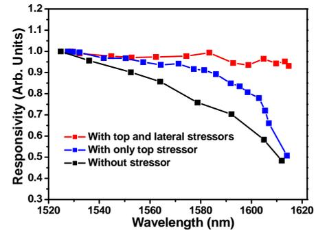
Fig. 9. Normalized responsivity of the devices with and without stressor scheme.
