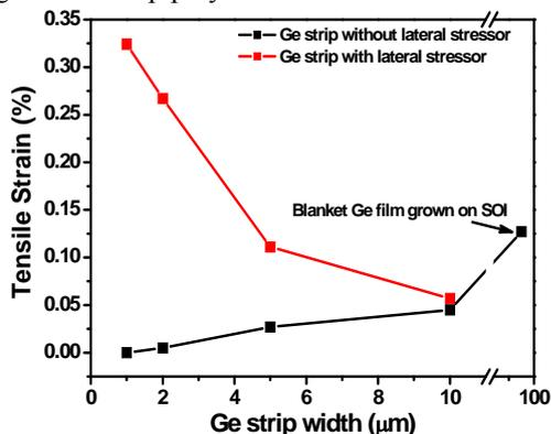
Fig. 8. In plane tensile strain in ge strip arrays for ge with and without SiN lateral stressors. The residue strain in blanket ge film grown on SOI is shown for reference.
