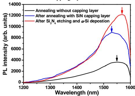
Fig. 5. PL spectra of the samples annealed without any capping layer (black), annealed with SiN capping layer (blue), and after SiN etching and a-Si deposition (red).
