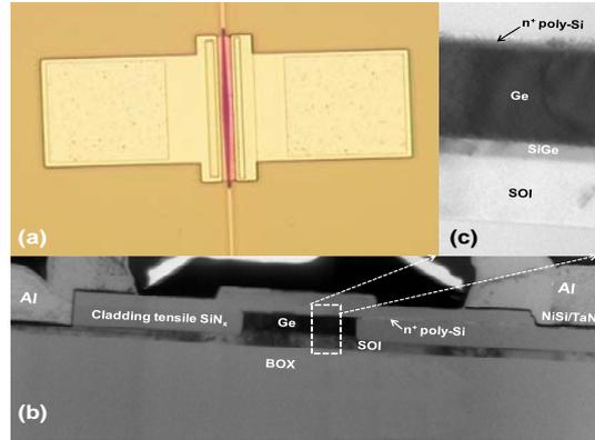
Fig. 6. (a) Top view micro-photograph of the fabricated device. (b) Cross sectional TEM images of the fabricated ge WGPD. (c) TEM image of active Ge region
