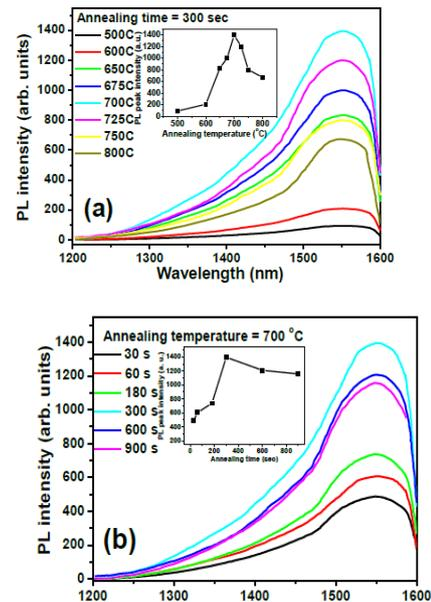
Fig. 2. (a) PL spectra for the  $n$ -doped Ge epi-films annealed at various temperatures for a fixed duration of 300 s. The inset shows the PL peak intensity as a function of annealing temperature. (b) PL spectra for the  $n$ -doped Ge epi-films annealed for various durations at a fixed temperature of 700 °C. The inset shows the PL peak intensity as a function of annealing time.
