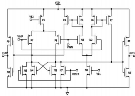
Fig. 4. Rail-to-rail latched comparator.
