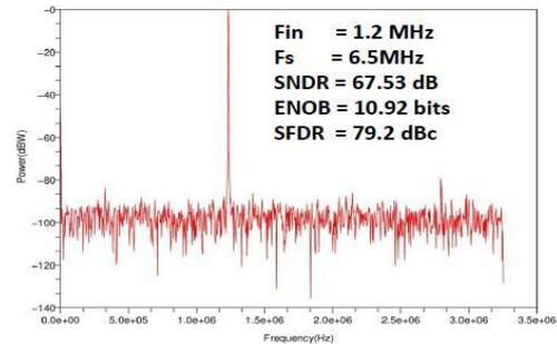
Fig. 6. Spectrum plot of the ADC.
