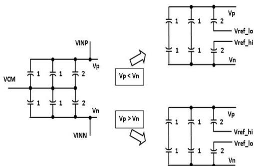
Fig. 3. Common mode resetting triple level switching scheme.
