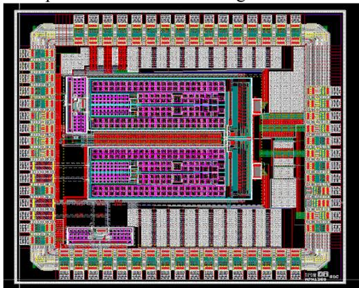
Fig. 5. Layout of the ADC test chip.
