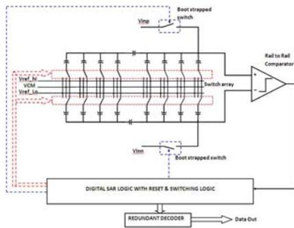
Fig. 1. Architecture of the proposed SAR ADC.
