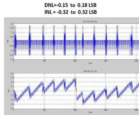
Fig. 7. Simulated DNL & INL plots of the ADC.
