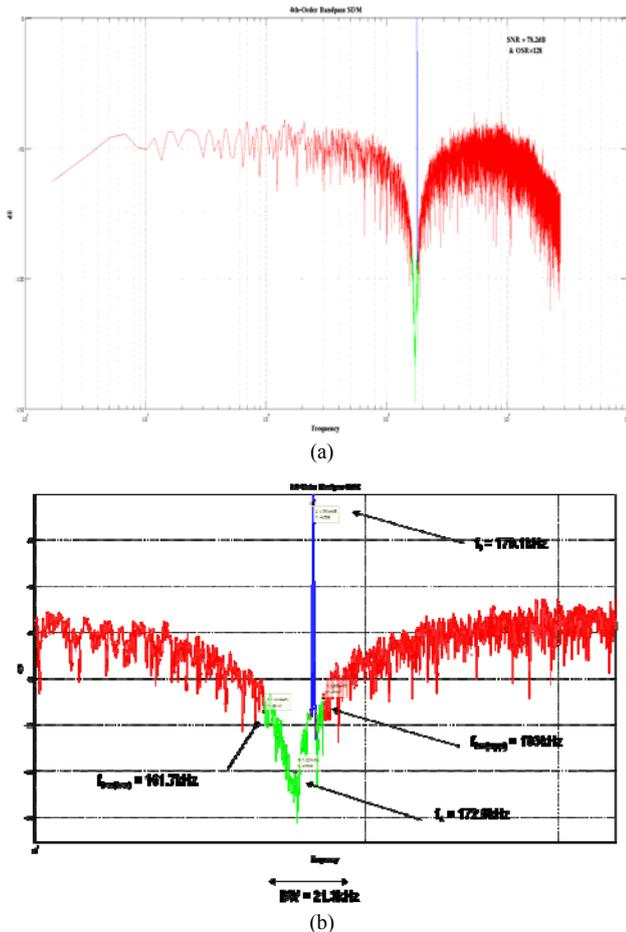
Fig. 4. (a) Simulated power spectrum density (32768-point FFT) plot with 179.1 kHz (0.5V<sub>pk-pk</sub>) input signal, (b) A zoom-in view.
