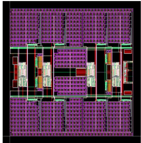
Fig. 5. Layout for the fully differential continuous-time bandpass delta-sigma modulator
