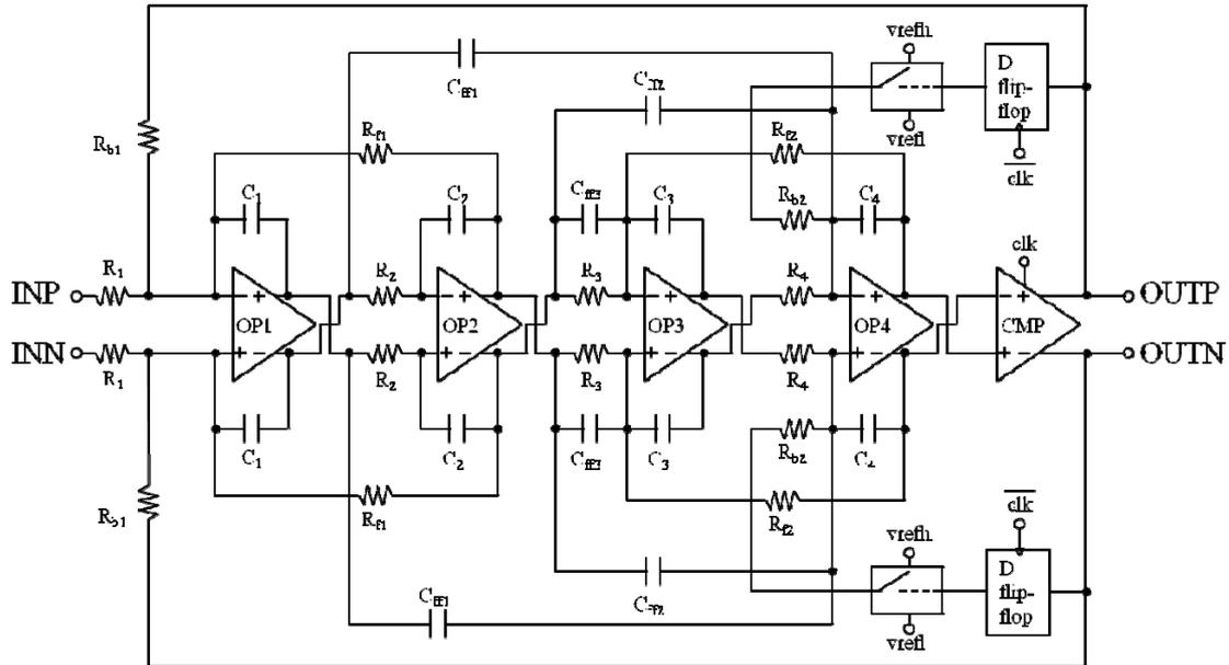
Fig. 3. Circuit implementation for the fully differential continuous-time bandpass delta-sigma modulator.
