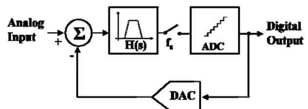
Fig. 1. Block diagram of continuous-time delta-sigma modulator.
