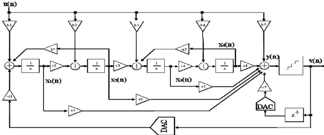
Fig. 2. Proposed system architecture for bandpass delta-sigma modulator
