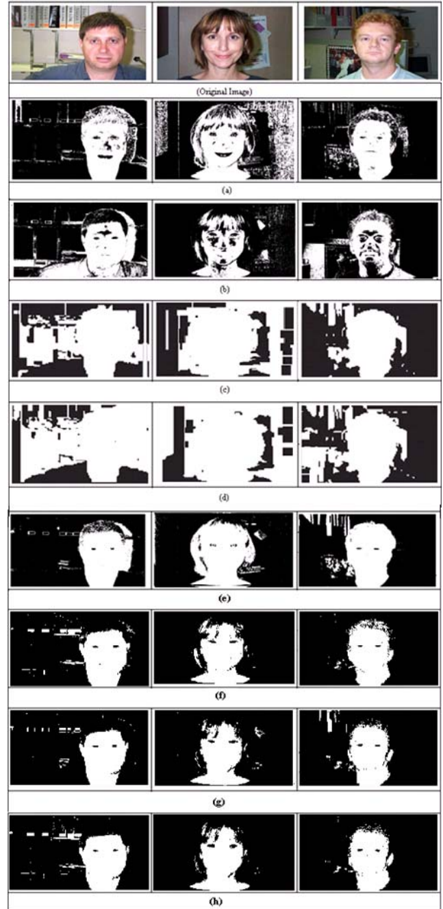
Fig. 1. Comparison of skin color segmentation results by different color models; (a) Normalized rg, (b) HSV, (c) YUV, (d) YIQ, (e) YCbCr, (f) RGB, (g) YCbCr-YU'V and (h) RGB-YU'V (proposed method) using CalTechDatabase
